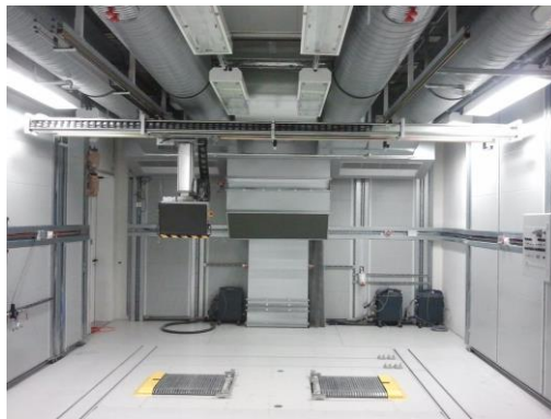
The monitor system can be moved anywhere in the entire test area.
